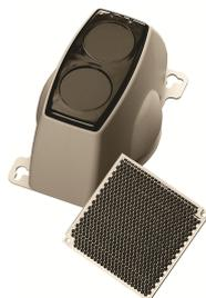
The Intelligent Reflective Beam Detector differs from a traditional beam detector in that it is a single unit which houses a transmitter, a receiver and the control electronics.
