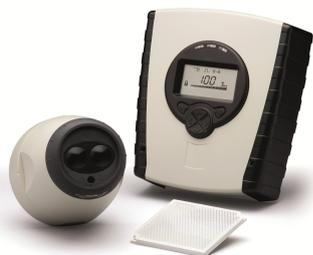
The high-performance Auto-Aligning Beam Detector comprises of a ground level controller, detector head with auto-aligning feature, integral laser for rapid initial alignment and single prism. An additional detector head can be added to the controller.
