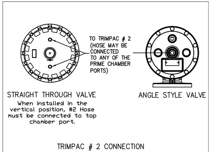
**Figure 11 - Valve Connections**
