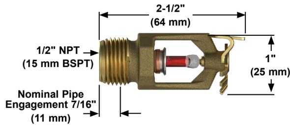
**Figure 2: Sprinkler Dimensions**
