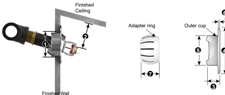
**Figure 5: Installation Dimensions with G-1 Escutcheon**
