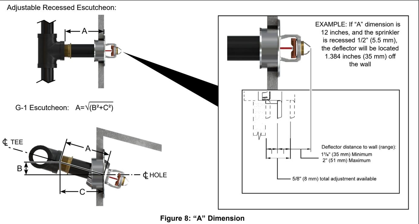
3. From below, choose a sprinkler base part number with the required thread size and listing or approval (refer to section 6).
