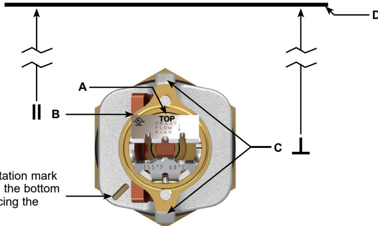
NOTE: Frame orientation mark must be oriented on the bottom left corner (when facing the sprinkler)
