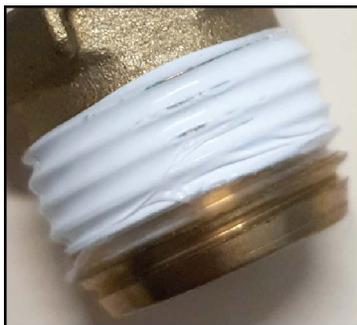
Figure – 3: Sealing the Threads
