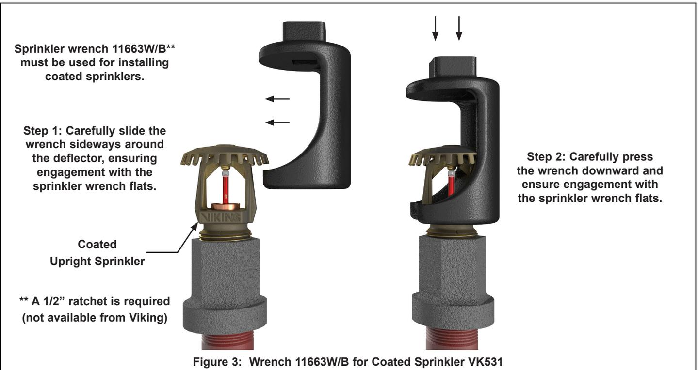
Figure 3: Wrench 11663W/B for Coated Sprinkler VK531
