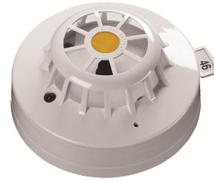
The XP95A Heat Detector monitors temperature by using a single thermistor which provides a voltage output proportional to the external air temperature. It is classified as an ordinary detector by UL. Well suited for warehouses, loading docks and parking areas
