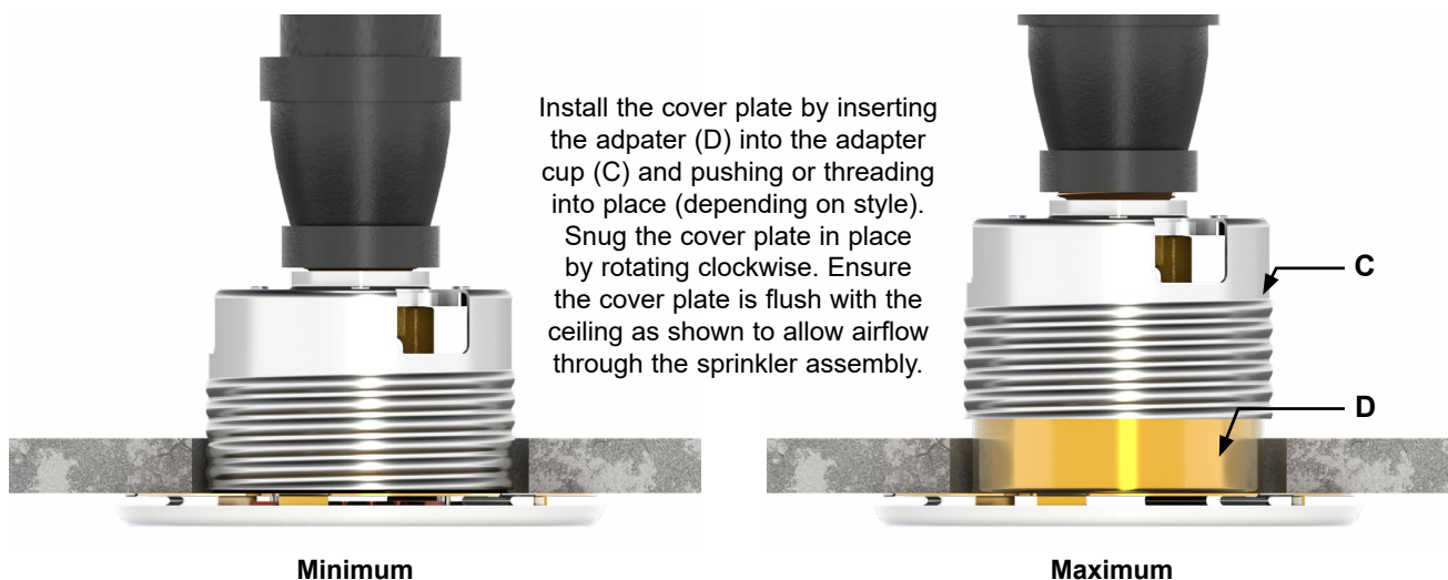
Figure 27: Installing the Cover Plate
