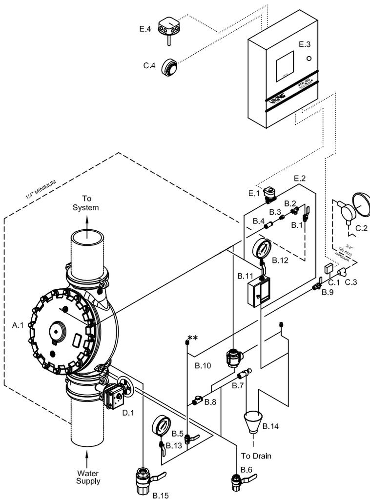
**FIGURE 8: STRAIGHT THROUGH DELUGE VALVE WITH CONVENTIONAL VERTICAL TRIM
