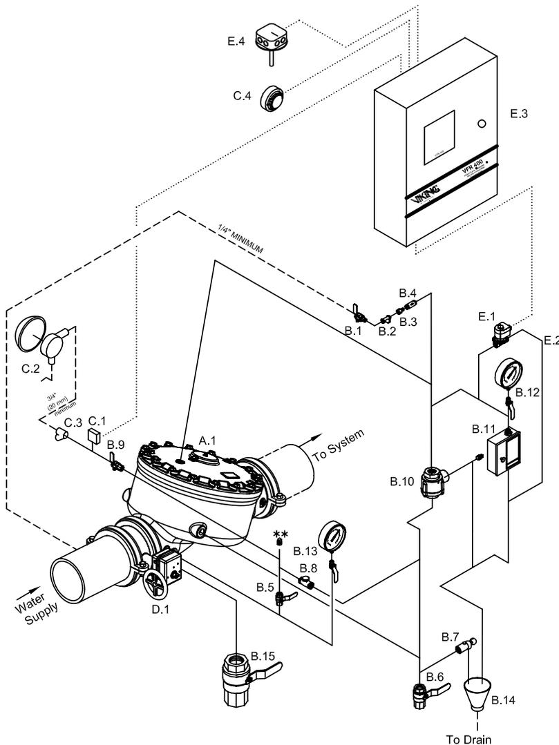
**FIGURE 3: STRAIGHT THROUGH DELUGE VALVE WITH HORIZONTAL CONVENTIONAL TRIM
